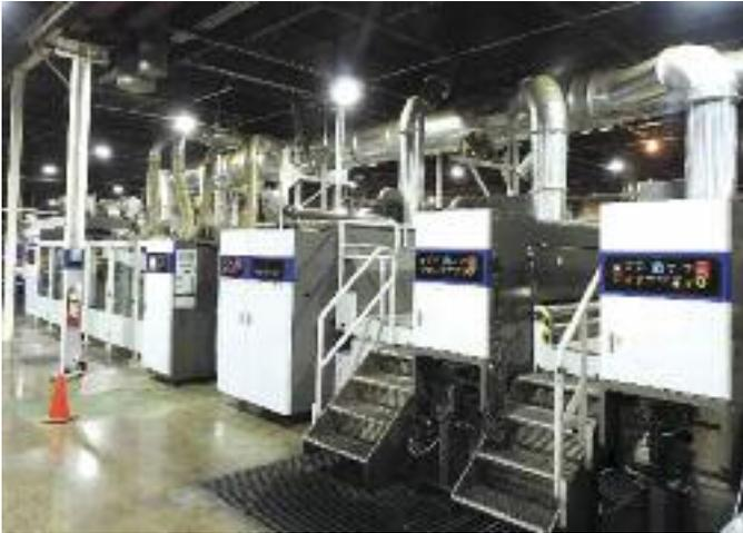
**MHI's Evol is a high-speed flexo folder-gluer that boasts fast set ups, quick ink changing and consistent stacking.**
